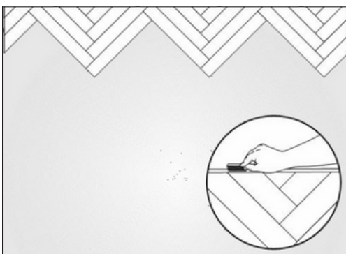
Figure 14: Put in spacers. Put in spacers between the flooring and the wall to ensure a expansion gap of 10/12 mm.
