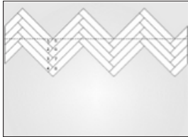
Figure 11: Number the panels from 1 to.... This will allow you to keep the panels in order. Dismantle the panels and cut them to size along the previous marked line.
